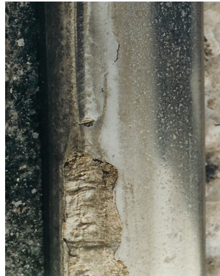
gauge-corner collapse in a well-lubricated rail
