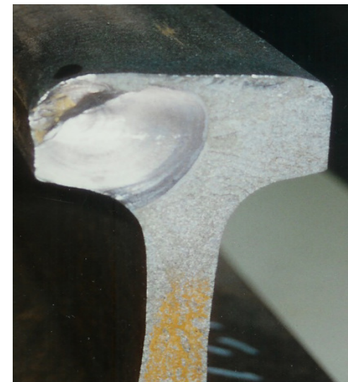
transverse defect from a shell.
