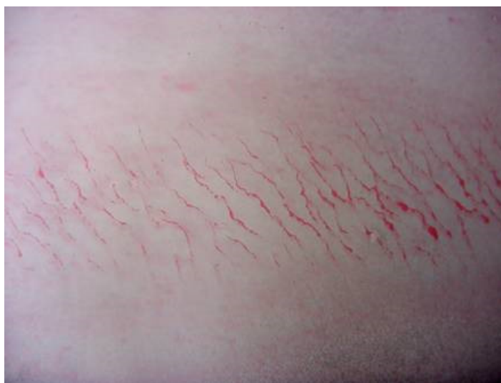
Micro-cracks on the field/rim side of the high-speed wheel.
