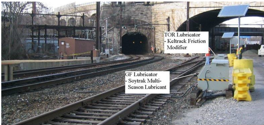
From P. Sroba et al, Testing of Rail Friction Management on the 377.2 Baltimore Curve, NRC report #54-A62209-T11-2-AUG05
