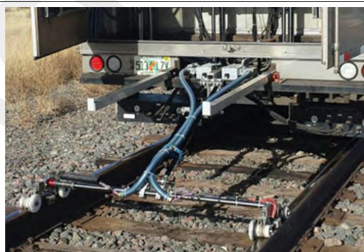
Rohman's hy-rail eddy current unit can have as many as 6 probes per rail. Running speeds are up to 40 mph.
